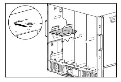
**4.** Push the device bay shelf back until it stops, lift the right side slightly to disengage the two tabs from the divider wall, then rotate the right edge downward (clockwise).
